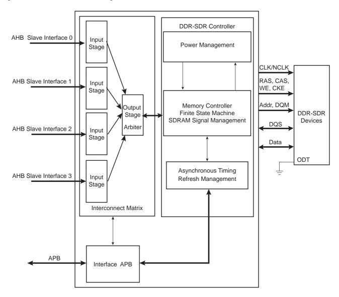
DDRSDRC is partitioned in two blocks (see Figure 21-1):
