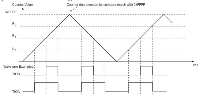
Figure 31-12. WAVSEL = 01 With Trigger
