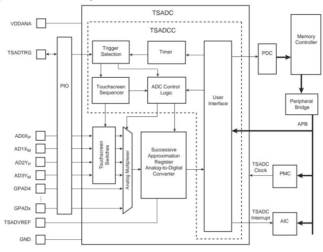
GPADx: last general-purpose ADC channel defined by the number of channels
