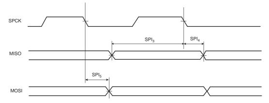
Figure 48-9. SPI Slave Mode 0 and 3)
