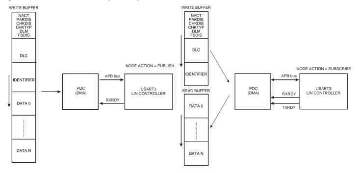
Figure 32-53. Master Node with PDC (PDCM = 0)
