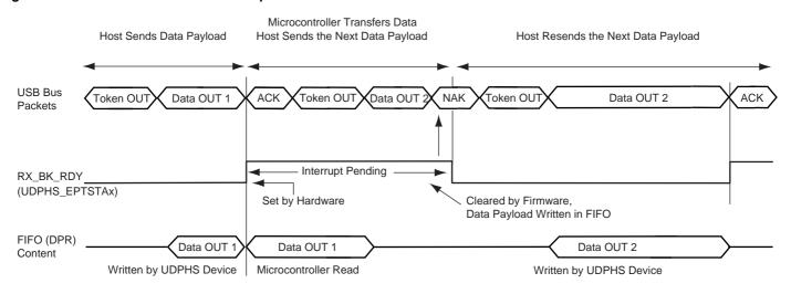
Figure 37-14. Data OUT Transfer for an Endpoint with Two Banks
