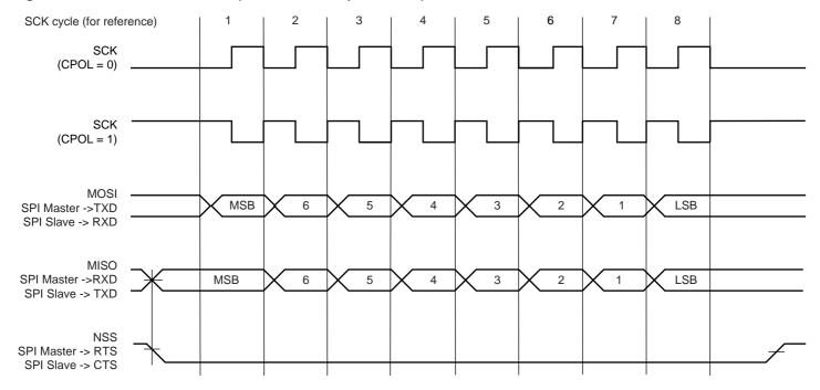
Figure 32-39. SPI Transfer Format (CPHA = 0, 8 bits per transfer)
