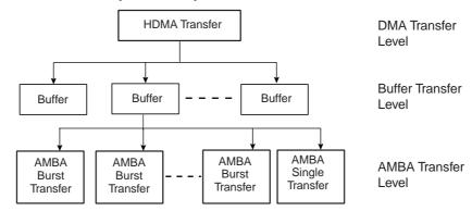
Buffer: A buffer of DMAC data. The amount of data (length) is determined by the flow controller. For transfers between the DMAC and memory, a buffer is broken directly into a sequence of AMBA bursts and AMBA single transfers.
