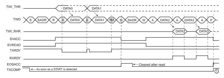
Note: 1. 1. TXCOMP is only set at the end of the transmission because after the repeated start, SADR is detected again.
