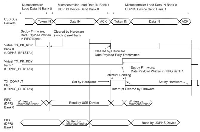
Figure 37-10. Data IN Followed By Status OUT Transfer at the End of a Control Transfer
