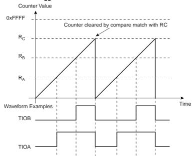
Figure 31-10. WAVSEL = 10 With Trigger
