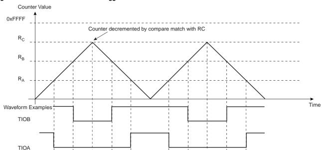
Figure 31-13. WAVSEL = 11 Without Trigger
