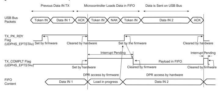
Figure 37-9. Data IN Transfer for Endpoint with Two Banks
