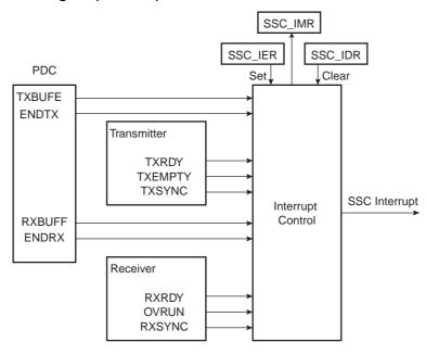
Figure 33-18. Interrupt Block Diagram (with DMA)
