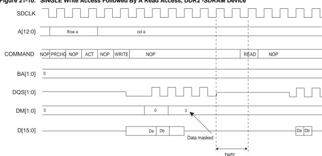
Figure 21-10. SINGLE Write Access Followed By A Read Access, DDR2 -SDRAM Device
