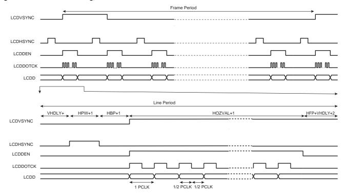
Figure 47-6. TFT Panel Timing, CLKMOD = 0, VPW = 2, VBP = 2, VFP = 1
