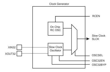
RCEN, OSC32EN, OSCSEL and OSC32BYP bits are located in the Slow Clock Configuration Register (SCKCR) located at address 0xFFFFD50 in the backed up part of the System Controller and so are preserved while VDDBU is present.
