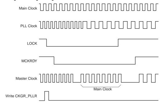
Figure 25-6. Programmable Clock Output Programming
