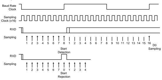
Figure 32-13. Asynchronous Character Reception
