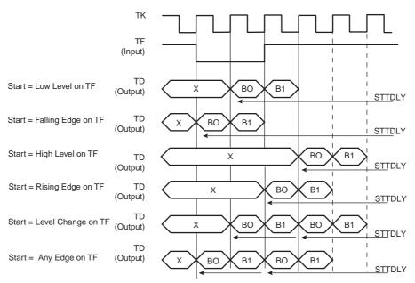
Figure 33-12. Receive Pulse/Edge Start Modes
