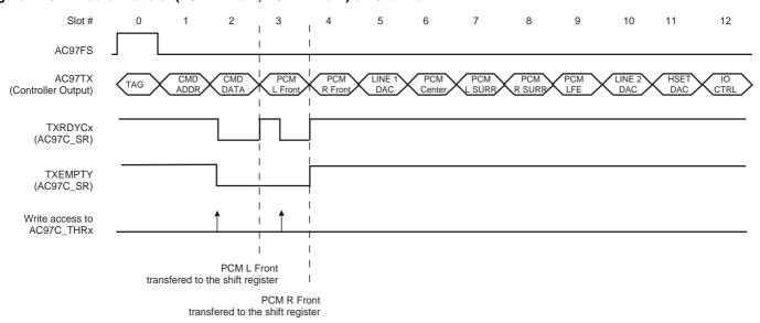
The TXEMPTY flag in the AC97 Controller Channel x Status Register (AC97C\_CxSR) is set when all requested transmissions for a channel have been shifted on the AC-link. The application can either poll TXEMPTY flag in AC97C\_CxSR or wait for an interrupt notice associated with the same flag.
