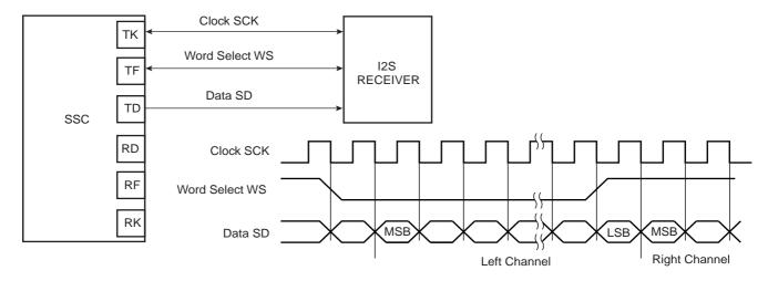
Figure 33-20. Codec Application Block Diagram
