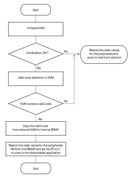
Figure 10-3. Remap Action after Download Completion
