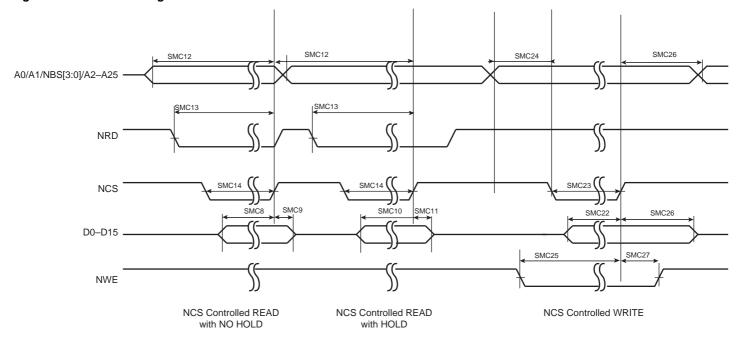
Figure 48-5. SMC Timings - NRD Controlled Read and NWE Controlled Write
