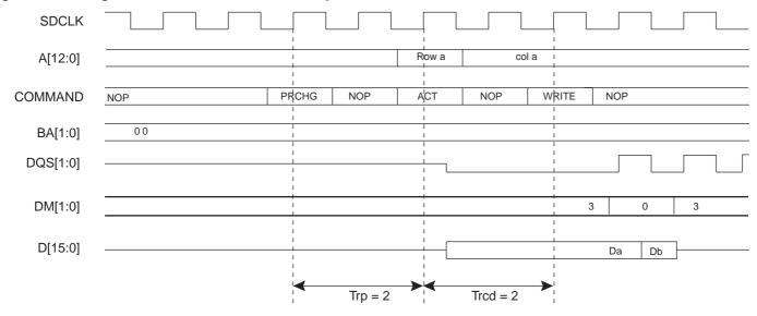
Figure 21-3. Single Write Access, Row Closed, DDR2-SDRAM Device
