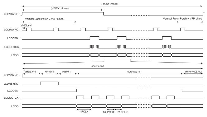
Figure 47-7. TFT Panel Timing (Line Expanded View), CLKMOD = 1
