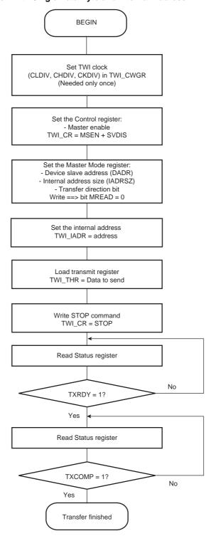
Figure 30-17. TWI Write Operation with Multiple Data Bytes with or without Internal Address
