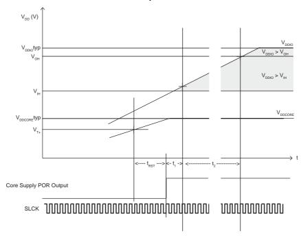
$V_{\text{DDCORE}}$  and  $V_{\text{DDBU}}$  are controlled by the internal PORs (Power-on Reset) to guarantee that these power sources reach their target values prior to the release of POR.
