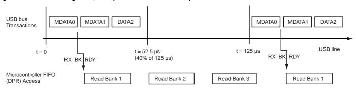
USB 2.0 supports individual High Speed isochronous endpoints that require data rates up to 192 Mb/s (24 MB/s): 3x1024 data bytes per microframe.
