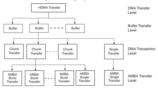
Figure 40-3. DMAC Transfer Hierarchy for Memory
