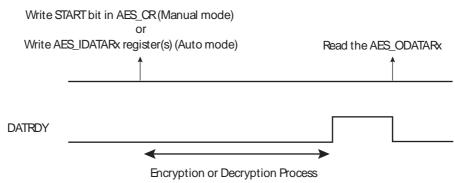
If the user does not want to read the output data registers between each encryption/decryption, the DATRDY flag will not be cleared. If the DATRDY flag is not cleared, the user cannot know the end of the following encryptions/decryptions.
