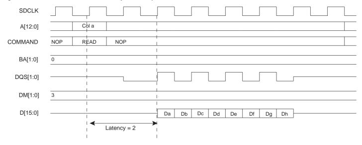
Figure 21-15. Burst Read Access, Latency = 3, DDR2-SDRAM Devices
