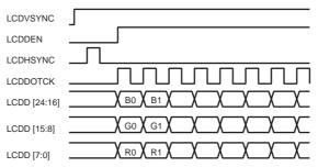
Figure 47-9. Single Scan Monochrome and Color 4-bit Panel Timing (First Line Expanded View)
