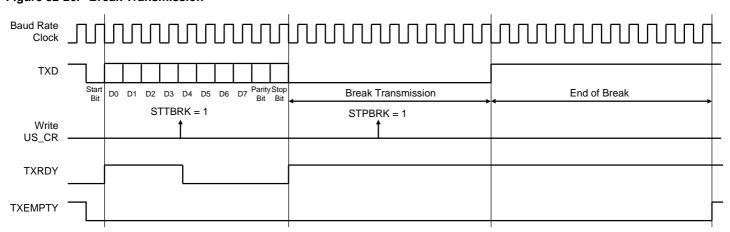
Figure 32-26. Break Transmission
