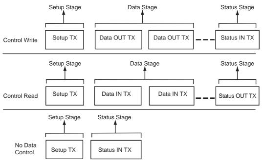
A status IN or OUT transaction is identical to a data IN or OUT transaction.
