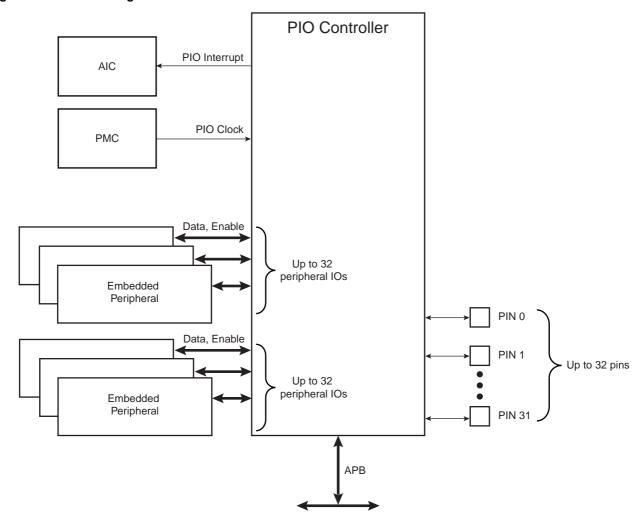
Figure 29-2. Application Block Diagram
