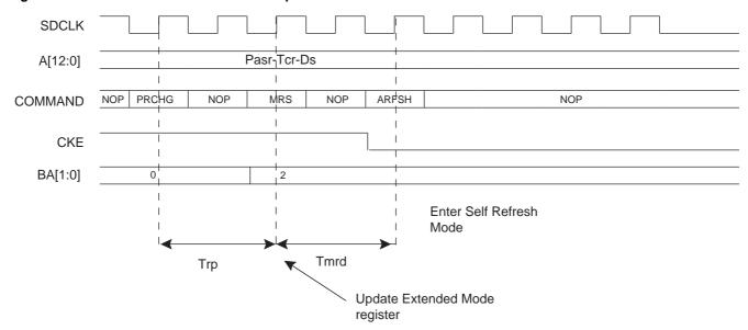
Figure 21-21. Automatic Update During AUTO-REFRESH Command and SDRAM Access
