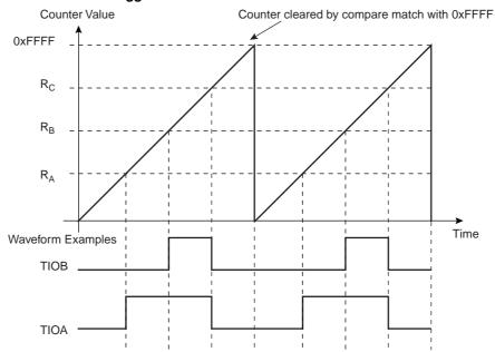
Figure 31-8. WAVSEL = 00 with trigger
