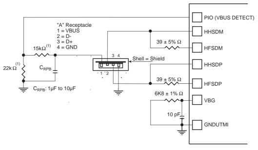
Note: 1. The values shown on the 22k  $\Omega$  and 15k  $\Omega$  resistors are only valid for 3v3 supplied PIOs.
