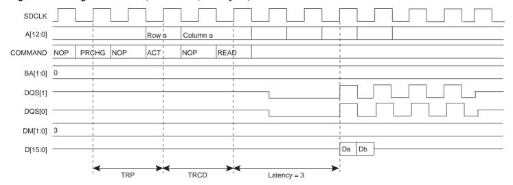
Figure 21-13. Single Read Access, Row Closed, Latency = 2, SDR-SDRAM Device
