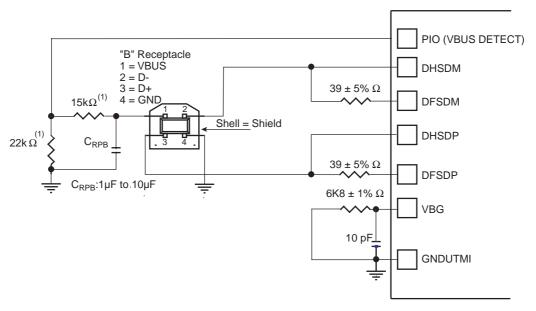
Note: 1. The values shown on the  $22k\Omega$  and  $15k\Omega$  resistors are only valid with 3V3 supplied PIOs.
