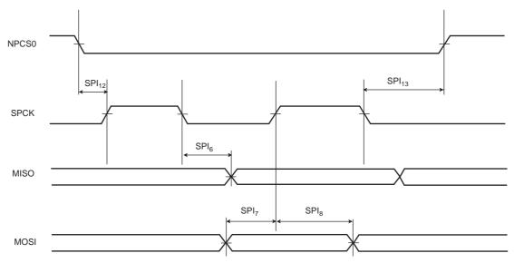
Figure 48-10. SPI Slave Mode 1 and 2
