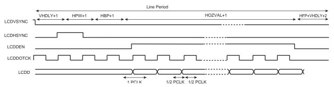
Usually the LCD\_FRM rate is about 70 Hz to 75 Hz. It is given by the following equation:
