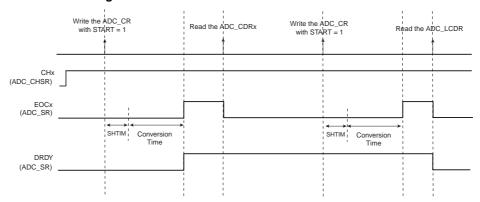
If the "TSADCC Channel Data Register x (x = 0..7)" is not read before further incoming data is converted, the corresponding Overrun Error (OVRE) flag is set in the "TSADCC Status Register".
