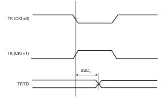
Figure 48-15. SSC Transmitter, TK in Output and TF in Input
