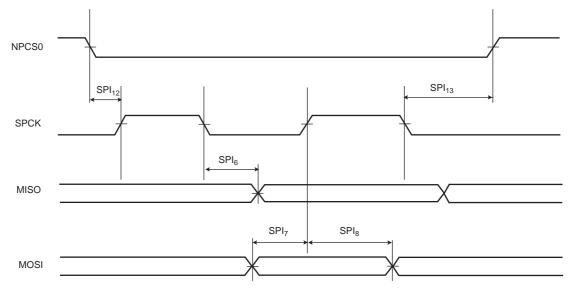
Figure 48-27. SPI Slave Mode - NPCS Timings
