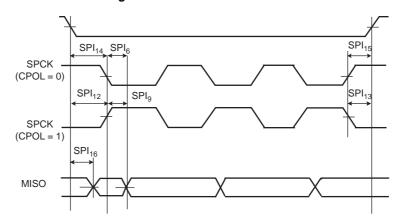
Table 48-34. SPI Timings with 3.3V Peripheral Supply
