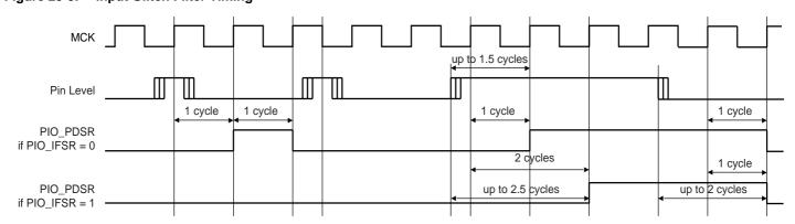
Figure 29-5. Input Glitch Filter Timing
