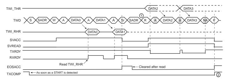
Notes: 1. In this case, if TWI\_THR has not been written at the end of the read command, the clock is automatically stretched before the ACK.
