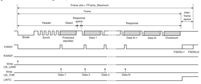
Figure 32-47. Master Node Configuration, NACT = SUBSCRIBE
