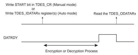
If the user does not want to read the output data registers between each encryption/decryption, the DATRDY flag will not be cleared. If the DATRDY flag is not cleared, the user will not be informed of the encryptions/decryptions that follow.
