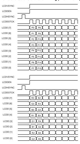
Figure 47-11. Dual Scan Monochrome and Color 8-bit Panel Timing (First Line Expanded View)
