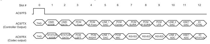
Table 42-4. AC-link Output Slots Transmitted from the AC97C Controller
