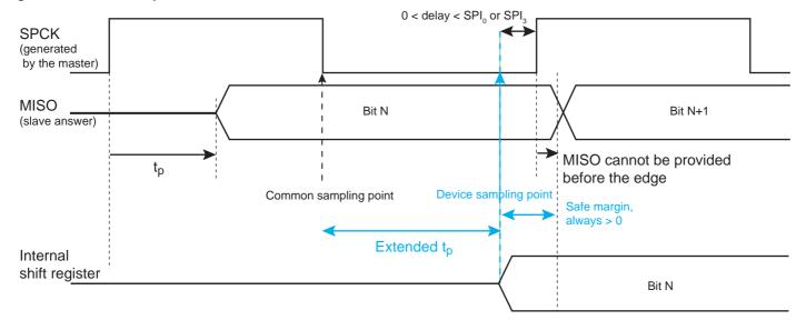
Figure 48-7. SPI Master Mode 1 and 2
