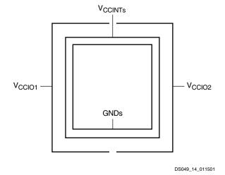
Figure 14: Split Rail V<sub>CC</sub> Output Power Connections in XC95144XV and XC95288XV Devices
