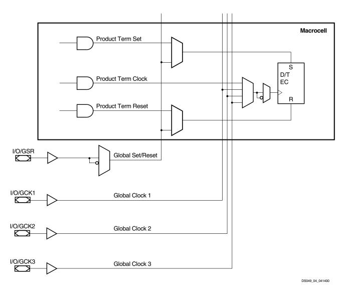
Figure 4: Macrocell Clock and Set/Reset Capability
