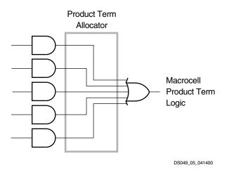
Figure 5: Macrocell Logic Using Direct Product Term
