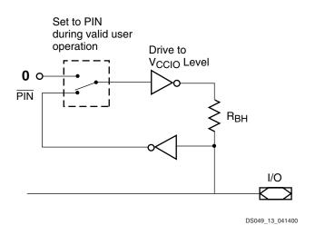
Figure 13: Bus-Hold Logic
