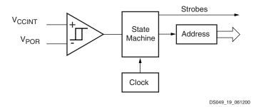
Figure 19: Configuration Controller
