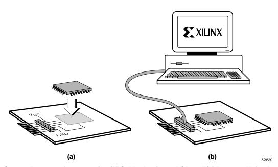
Figure 15: In-System Programming Operation (a) Solder Device to PCB and (b) Program Using Download Cable
