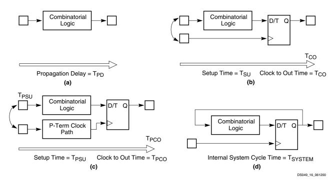
Figure 16: Basic Timing Model
