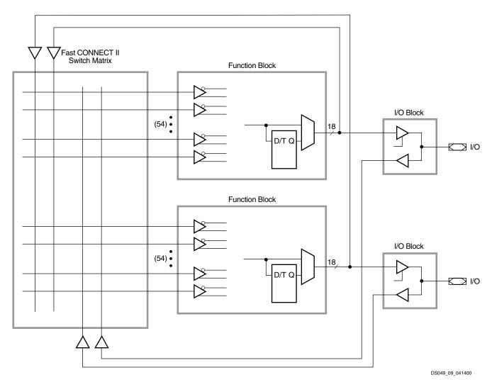
Figure 9: Fast CONNECT II Switch Matrix
