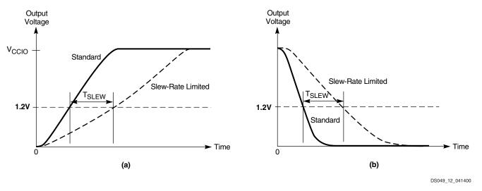
Figure 12: Output Slew-Rate Control For (a) Rising and (b) Falling Outputs
