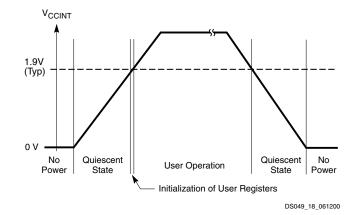
Figure 18: Device Behavior During Power-up
