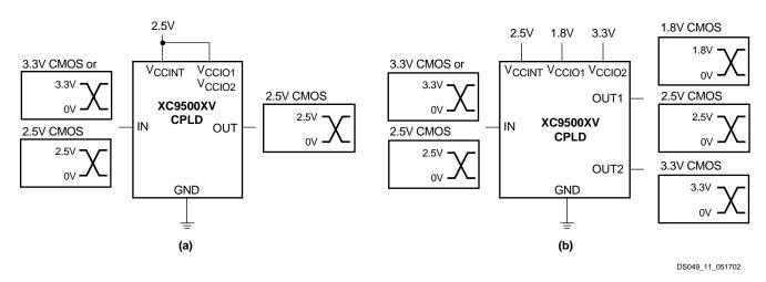
Figure 11: XC9500XV Devices in (a) 2.5V only and (b) Mixed 3.3V/2.5V/1.8V Systems
