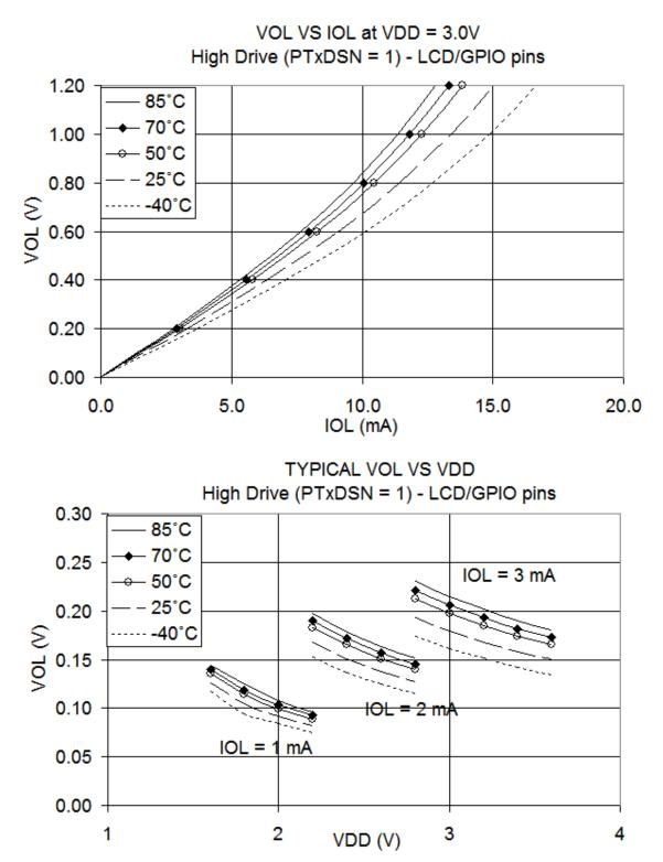
Figure 10. Typical Low-Side Driver (Sink) Characteristics (LCD/GPIO Pins) — High Drive (PTxDSn = 1)
