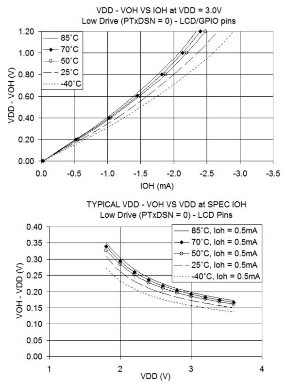
Figure 11. Typical High-Side (Source) Characteristics (LCD/GPIO Pins)— Low Drive (PTxDSn = 0)
