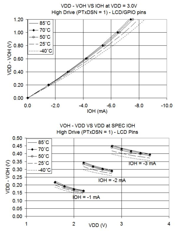
Figure 12. Typical High-Side (Source) Characteristics (LCD/GPIO Pins) — High Drive (PTxDSn = 1)
