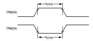
Figure 20. Timer Input Capture Pulse
