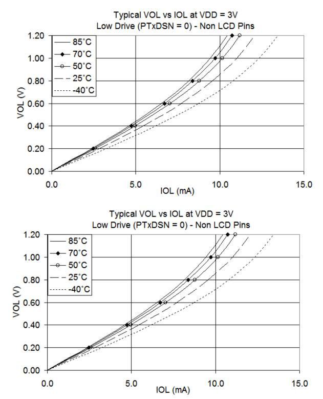
Figure 5. Typical Low-Side Driver (Sink) Characteristics (Non LCD Pins) — Low Drive (PTxDSn = 0)
