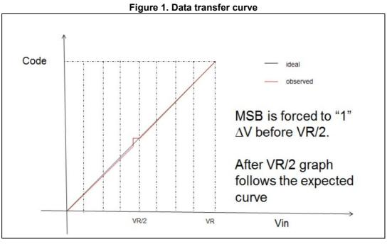
Note: The transfer curve behaves as expected when  $V_{IN}$  is strictly lower or higher that  $V_{REF+}/2$ .
