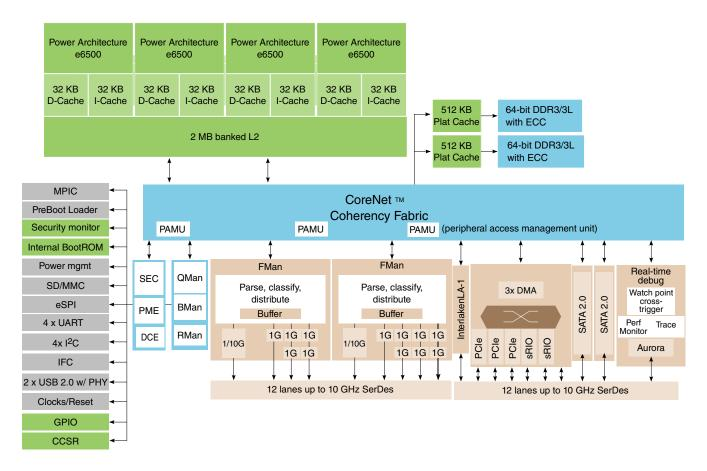
Figure B-1. T4080 block diagram
