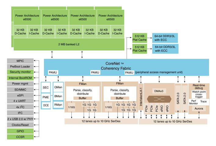
Figure A-1. T4160 block diagram
