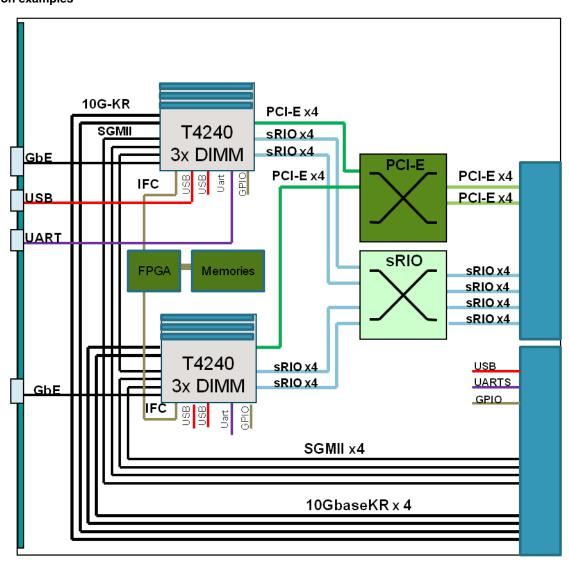
Figure 3. Radio node controller
